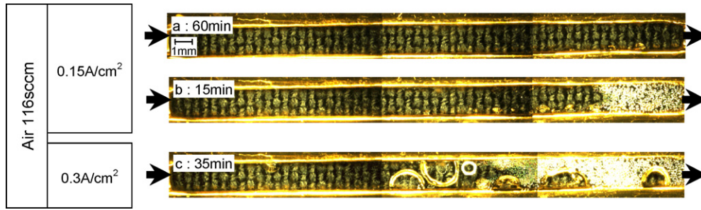
Fig. 8. Images of cathode GFC at the specified time, under the air flow rate condition of 116 sccm, with the different current: 0.3 A cm -2 (No. 2-2); 0.15 A cm -2 (No. 1-2).
